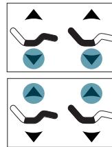
Press and hold the HEAD DOWN and FOOT DOWN buttons together for three (3) seconds, then hold HEAD UP and FOOT UP for three (3) seconds until the remote backlight flashes twice.
